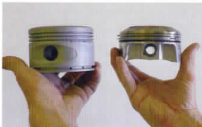
Factory 7:1 compression ratio O-200 piston on the left, Pete's custom 9:1 short-skirt piston on the right.
