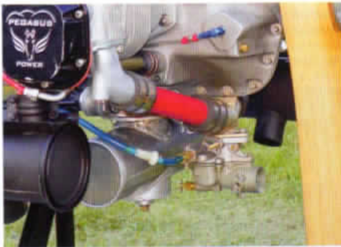
The prototype's welded-aluminum oil tank can be seen just behind the Zenith carb that was used for testing only.
