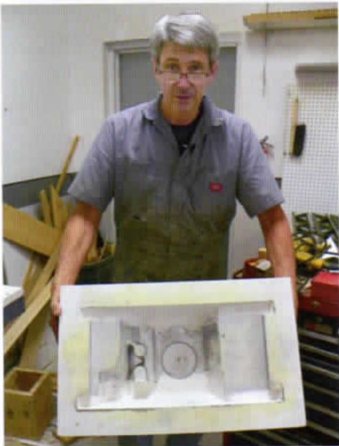
Pete Plumb at his shop in Shafter CA, showing the pattern for casting the inside of the crankcase.
